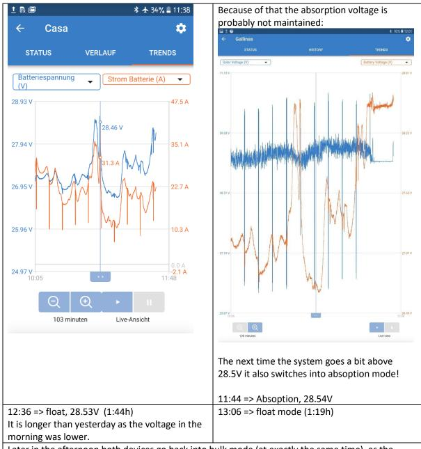
Later in the afternoon both devices go back into bulk mode (at exactly the same time), as the voltage drops below 26V, because the battery is now delivering Power.
