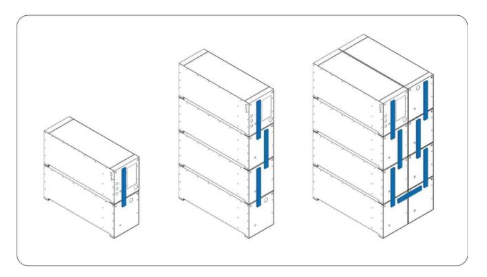
Connect the enclosures in serie: B1(+) to B2(-); B2(+) to B3(-); B3(+) to B4(-) etc. as illustrated.
