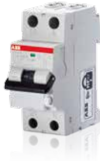
DS201 Type F , compact RCBO 1P+N with rated current 6...40A, B/C curves and breaking capacity 10kA in only two modules.
