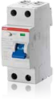
F202 Type F , RCCB in two poles with rated current 25-40-63A and sensitivity 30mA for the protection of single phase circuits.
