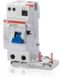
DDA 202 Type F , RCD blocks (to be mounted with S202 MCBs) in two poles with rated current 40 and 63A and sensitivity 30mA for quick and flexible solutions.
