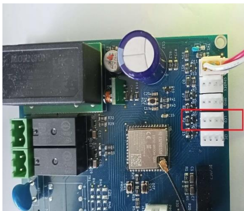
Picture 5 - Wires are disconnected from the PCB
