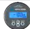
BMV-700 Battery Monitor The BMV-700 Battery Monitor features an advanced microprocessor control system combined with high resolution measuring systems for battery voltage and charge/discharge current. Besides this, the software includes complex calculation algorithms, like Peukert's formula, to exactly determine the state of charge of the battery. The BMV-700 selectively displays battery voltage, current, consumed Ah or time to go. The monitor also stores a host of data regarding performance and use of the battery. Several models available (see battery monitor documentation).
