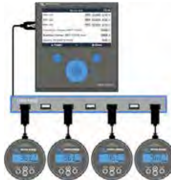
A maximum of four BMVs can be connected directly to the Color Control. Even more BMVs can be connected to a USB Hub for central monitoring.
