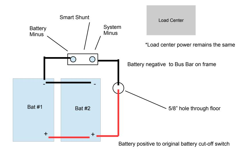
Relocating batteries to pass-through. Purchasing slightly longer 8 awg wires and routing them through The 5/8" hole in the floor. The positive going to the original cut-off switch. The negative going to the bus Bar on the frame. \*Power to the load center comes from the second terminal on the cut-off switch.
