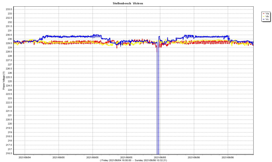
Graph Showing the Voltage profiles with a 1minute average measured at the DB Board away from the inverter
